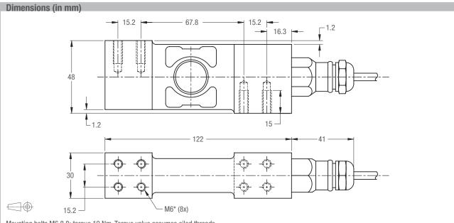
Mounting bolts M6 8.8; torque 10 Nm. Torque value assumes oiled threads.  $^{\star}$  Unified thread 1/4-20 UNC is available.
