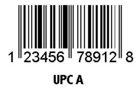
UPC-A has two variations (UPC-A Plus 2 and Plus 5) which increase the amount of information contained. They add either 2 or 5 digits in a second, smaller bar code following the first.
